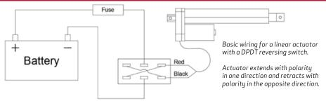
**Note:** If you are using one of our industrial actuators (black in color) that has limit switches built into it, do not let the extension shaft rotate when it is extending or retracting. Doing so can allow the limit switches to move out of adjustment which could reduce the usable length of stroke.
